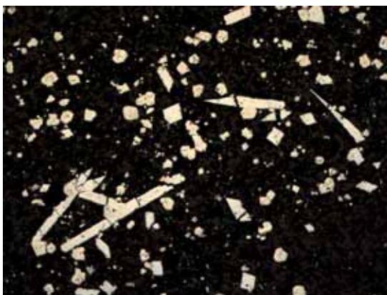
Photomicrograph showing arsenopyrite needles with cubic pyrite in sandstone. LODH004, 225.1m, assay grade at 41 g/t gold over approximately 1m interval.
