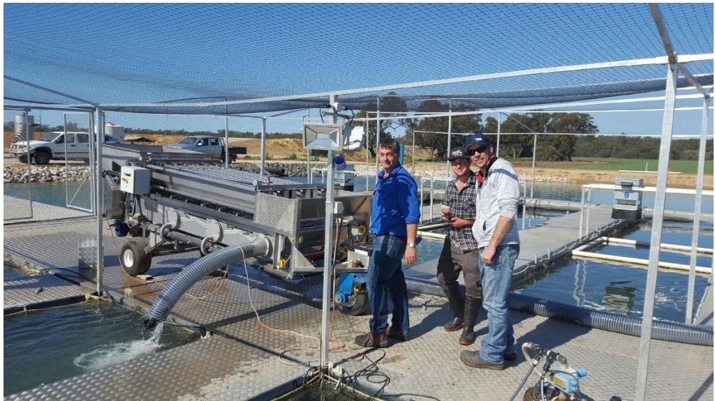
Picture 6: Fish grading machine operating on contract grower farm
