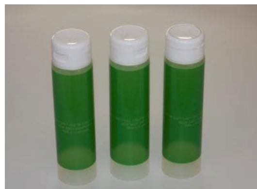
Thin wall extruded tubes made from Cardia Biohybrid™
