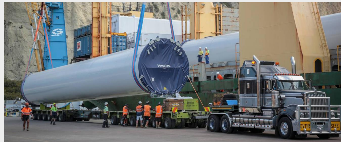
Turbine tower sections unloading at Napier Port
