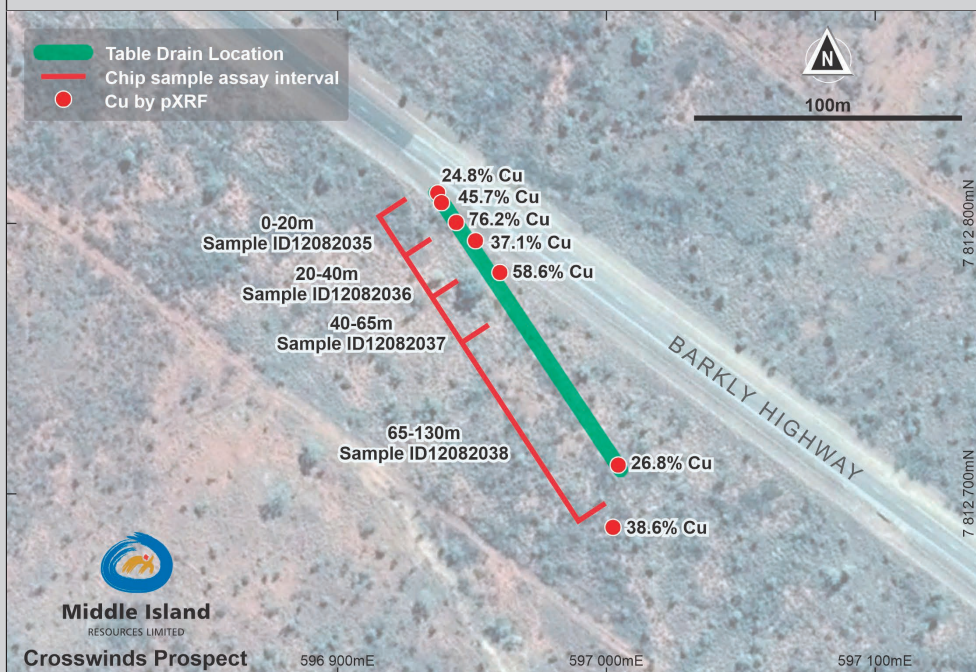
Figure 3. Crosswinds Copper Prospect – Plan of chip sampling traverse and pXRF results.
