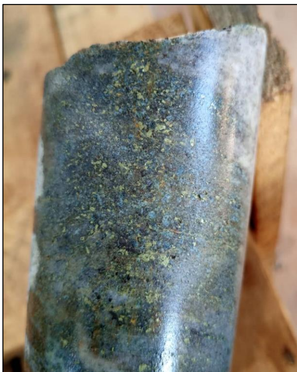
Figure 3 – Detail from CKDD003 (36m) exhibiting silicified metagranodiorite with up to 3% visually logged disseminated chalcopyrite
