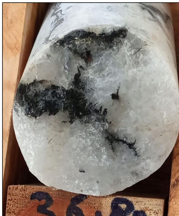
Figure 4 – Detail from CKDD002 at 37m showing tourmaline-pyrite mineralisation within quartz vein zone
