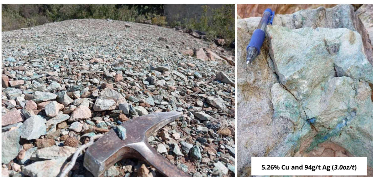
Figure 4 – Mina Emilia waste dump (left) and outcrop (right) where sample 171-01-01 was collected. Outcrop shows copper oxide mineralisation (green and blue minerals).
