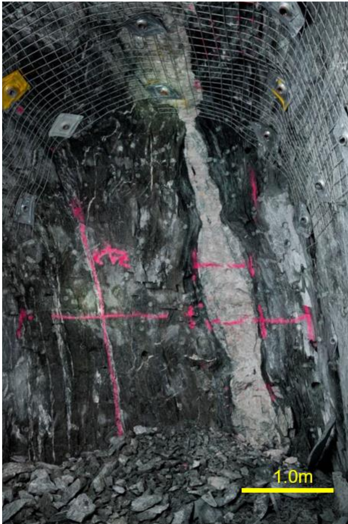
Figure 9: Photo of the high-grade Wilber lode in underground development at Andy Well showing the laminated hydrothermal quartz vein, and pinching and swelling nature of the mineralisation.
