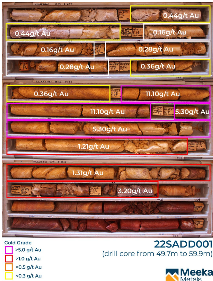
Figure 6: Diamond core from 22SADD001 showing alteration zone and high-grade gold interval of 7.8m @ 2.69g/t Au from 50.2m including 2.0m @ 8.20g/t Au.
