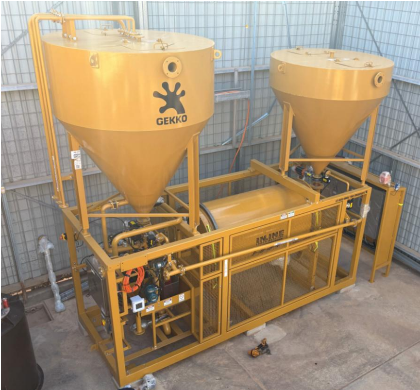
Figure 5: Installation of the InLine Leach Reactor (ILR), part of the gravity gold circuit, in the gold room, April 2025.
