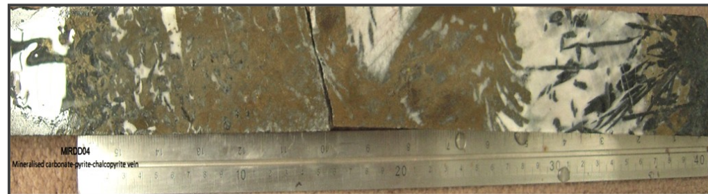
Example of copper mineralisation (chalcopyrite) observed in Miranda drill hole MIRDD01 and MIRDD04.
