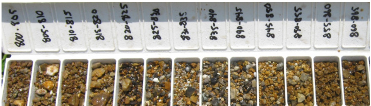
Figure 3(c): Significant gold mineralised intersection of 6.10m at 2.09 g/t Au (using 0.5 g/t Au lower cut) from 815-835ft (248.41 – 254.51m) within broader anomalous interval reporting 27.43m at 0.65 g/t Au in AW12-08. Mineralisation is laterally dispersed and is associated with silica flooding along the Tertiary conglomerate – Triassic limestone interface at 820ft (250m). Note last appearance of rounded rhyolite clasts extend the conglomerate to 820ft.
