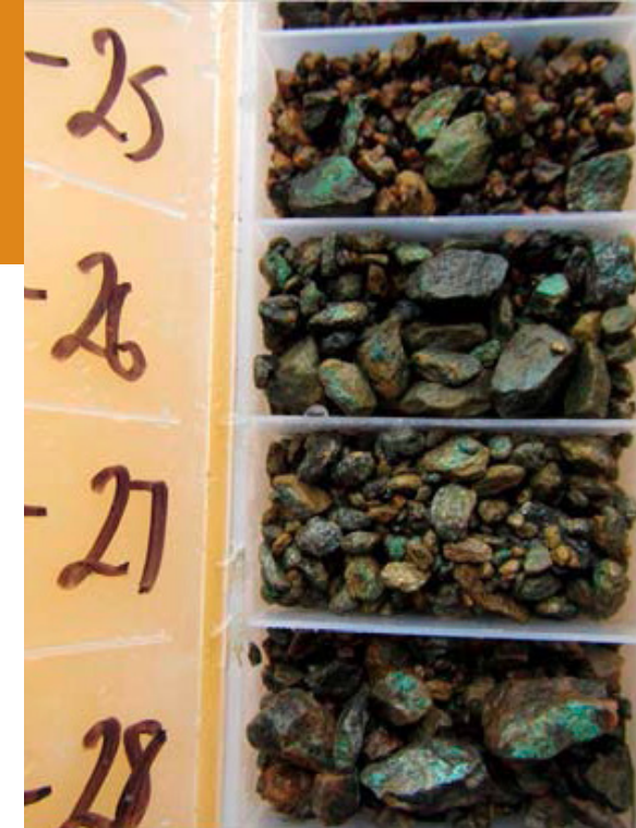
Example of malachite logged in Phase 1 drill hole WMAC007.
