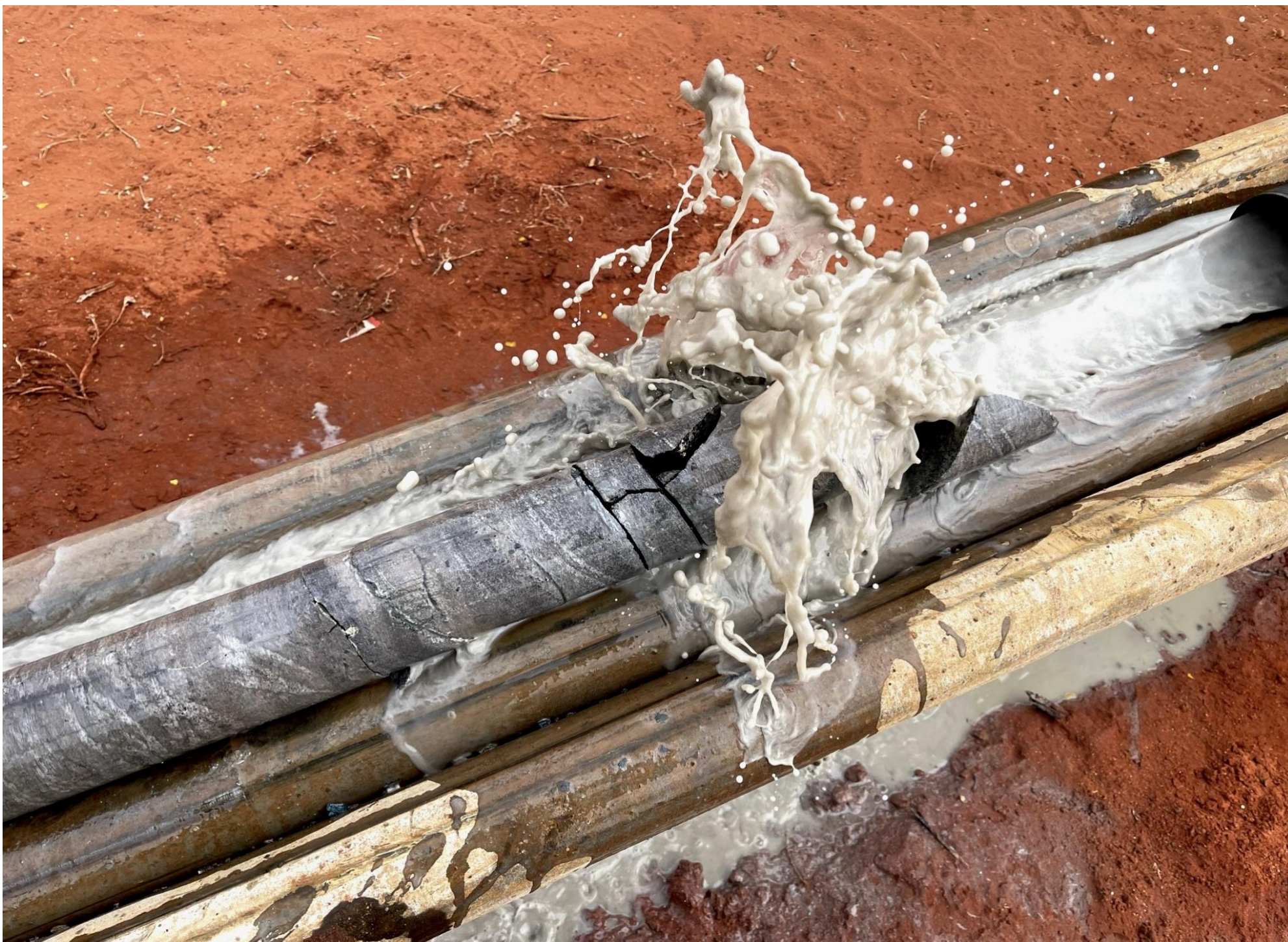
Figure 1: Diamond core being pumped out of the drilling rods at Aurora Tank (May 2023)
