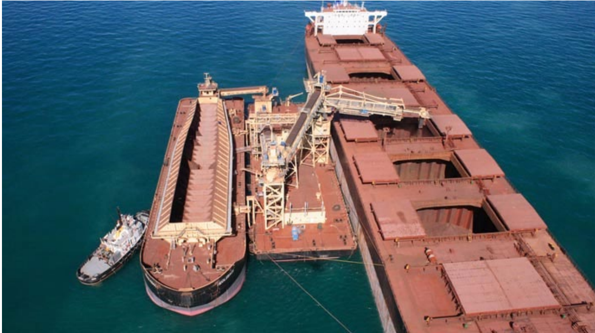
Figure 3. Transshipping offloading at anchorage into Capesize vessel in Spencer Gulf
