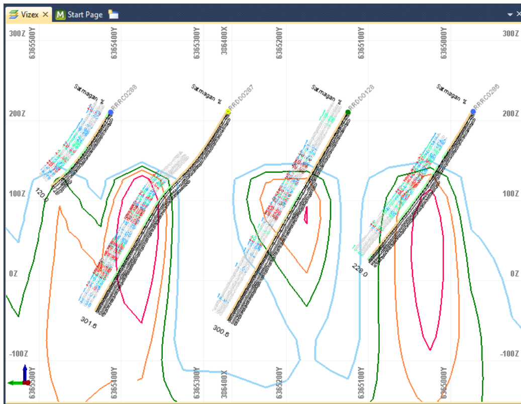
Figure 15: Cross-Section of Dragons Head drill line, with magnetic shells. While the model shells show very high magnetic susceptibility, the drilling failed to meet the same expectation. 3D shells: 0.1 SI unit cutoff – Blue; 0.25 SI unit cutoff – Green; 0.4 SI unit cutoff – Orange; 0.6SI unit cutoff – Red
