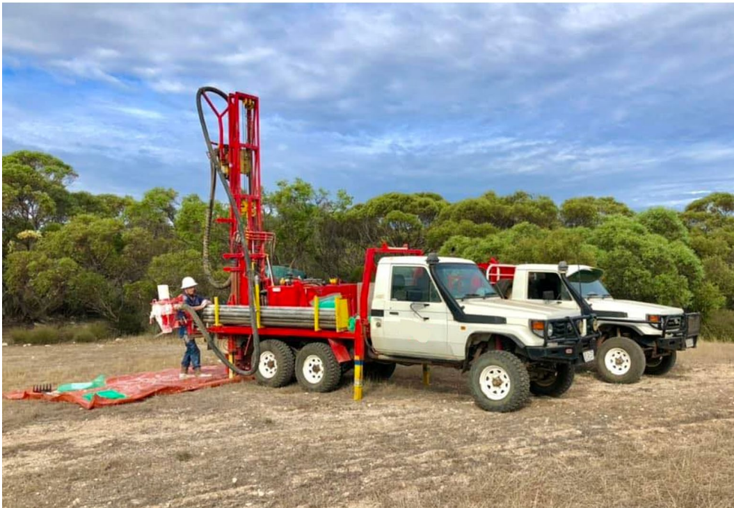
Figure 2. Typical 4WD mounted air core drilling rig.
