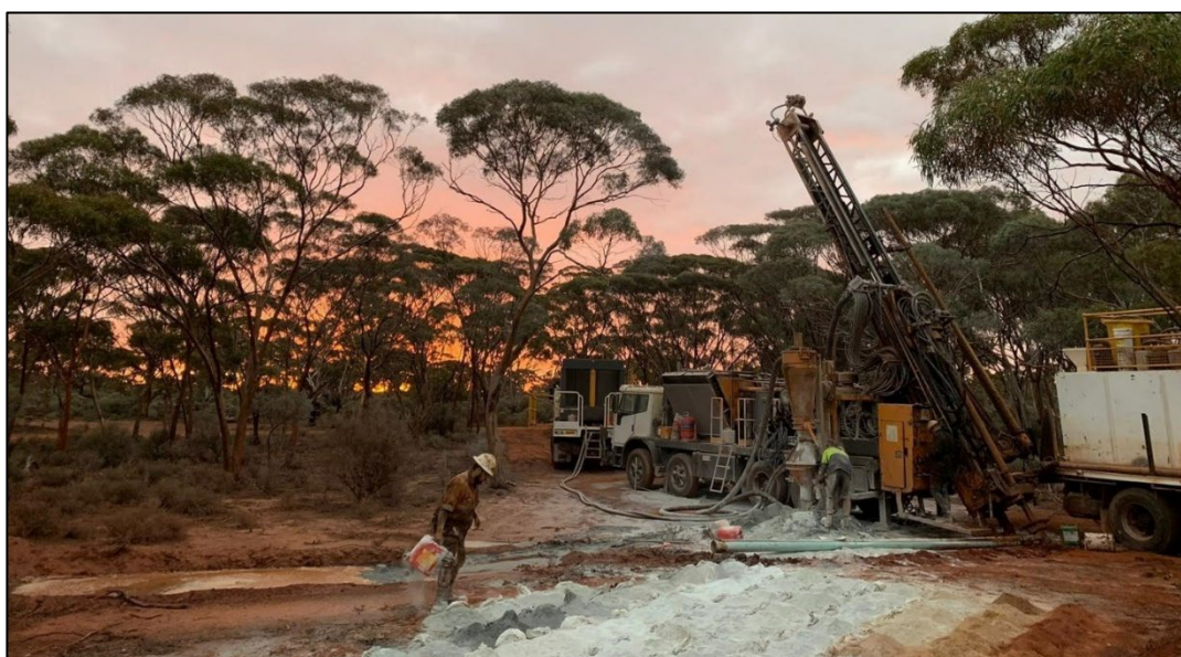
Figure 3. RC drilling at Berehaven
