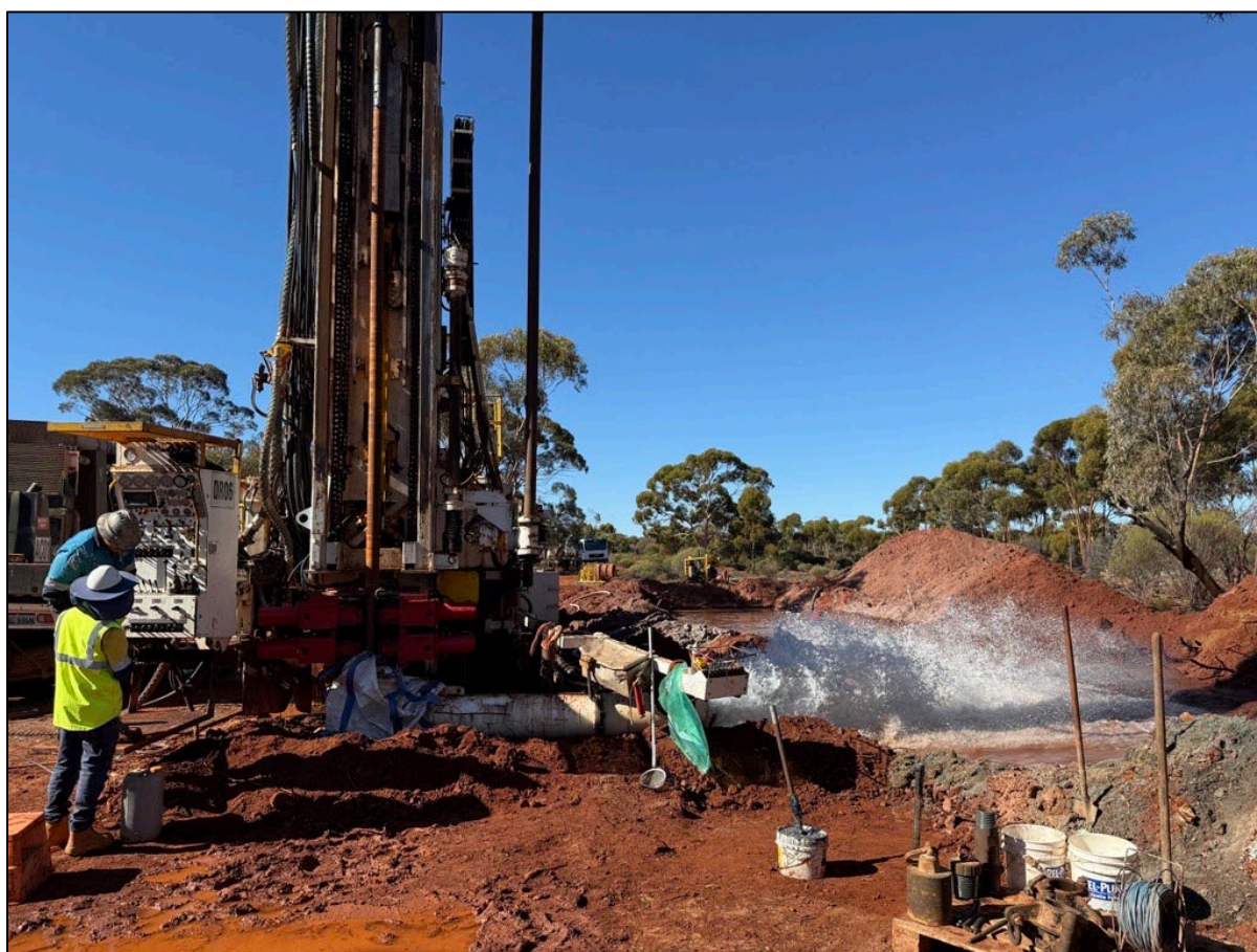
Figure 2: Water bore airlift testing
