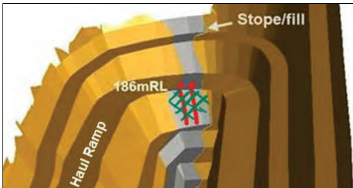
Figure 16-1 View looking south showing support for stope fill crossed by haul ramp at southern end of pit
