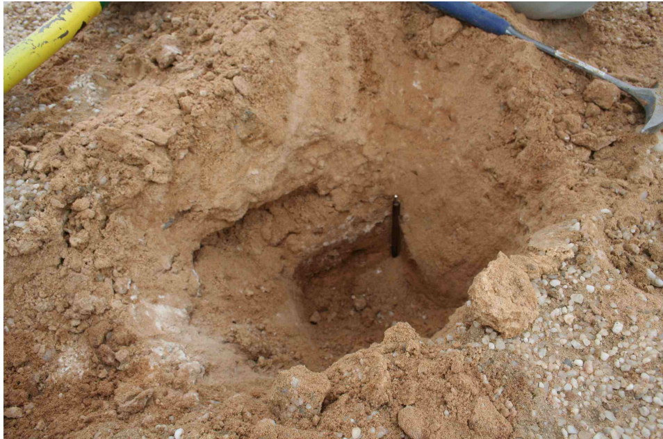
Trial pit at Kudu South yielding 0.53% U 3 O 8 in the top 50 cm and 2.31% U 3 O 8 at depth.
