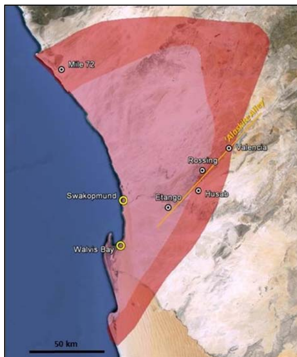
Figure 2 – Areas exhibiting prime geological conditions for the genesis of alaskites. Mile 72 has the same conditions as those experienced at Husab, Rössing and Valencia. (Red = peak conditions ideal for genesis of alaskite. Pink = peak conditions exceeded required conditions but area still hosts potential for alaskites.)
