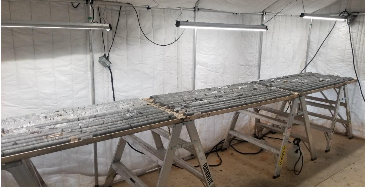
Figure 8: Drill core of DDH LR19-09 which intersected the Graphitic Carheil Zone over an extensive thickness of 75.2m (apparent thickness) from a depth of 9.5m to 84.7m
