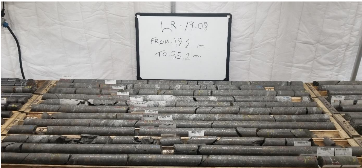
Figure 9: Drill core of DDH LR19-08 which intersected a zone of semi-massive graphite mineralisation corresponding with the Main Graphitic Carheil Zone. The drill core shown in the image represents an intersection of 17.0m (apparent thickness) from a depth of 18.2m to 35.2m, which is contained within a larger intersection of 47.72m (apparent thickness) from a depth of 7.83m to 55.5m
