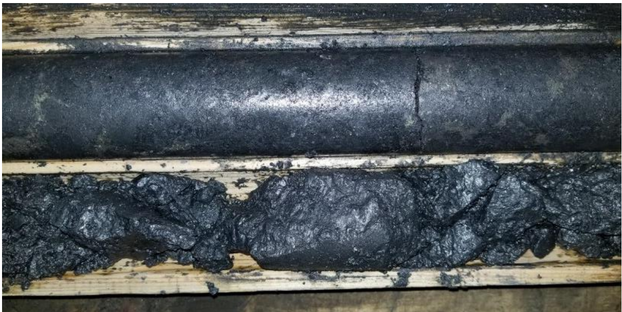
Figure 6: Close-up of the main graphitic zone encountered in DDH LR19-05, illustrating a solid drill core graphite intersection ( top of core box ) and a fractured / broken graphite intersection ( bottom of core box ), Lac Rainy Graphite Project
