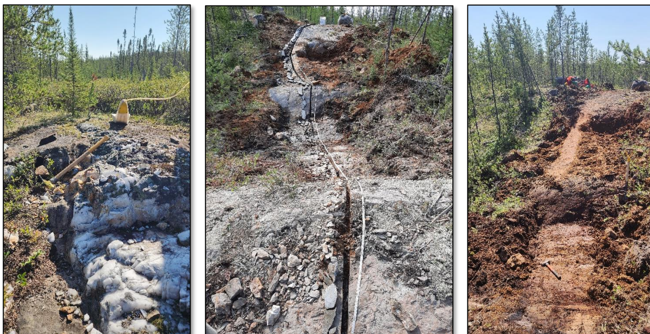
Photo 9, 10, 11 (L → R): Western side of East Eade: Quartz Vein – Historic sample location, Diamond cutting through outcrop & Trenching preparation for CV24
