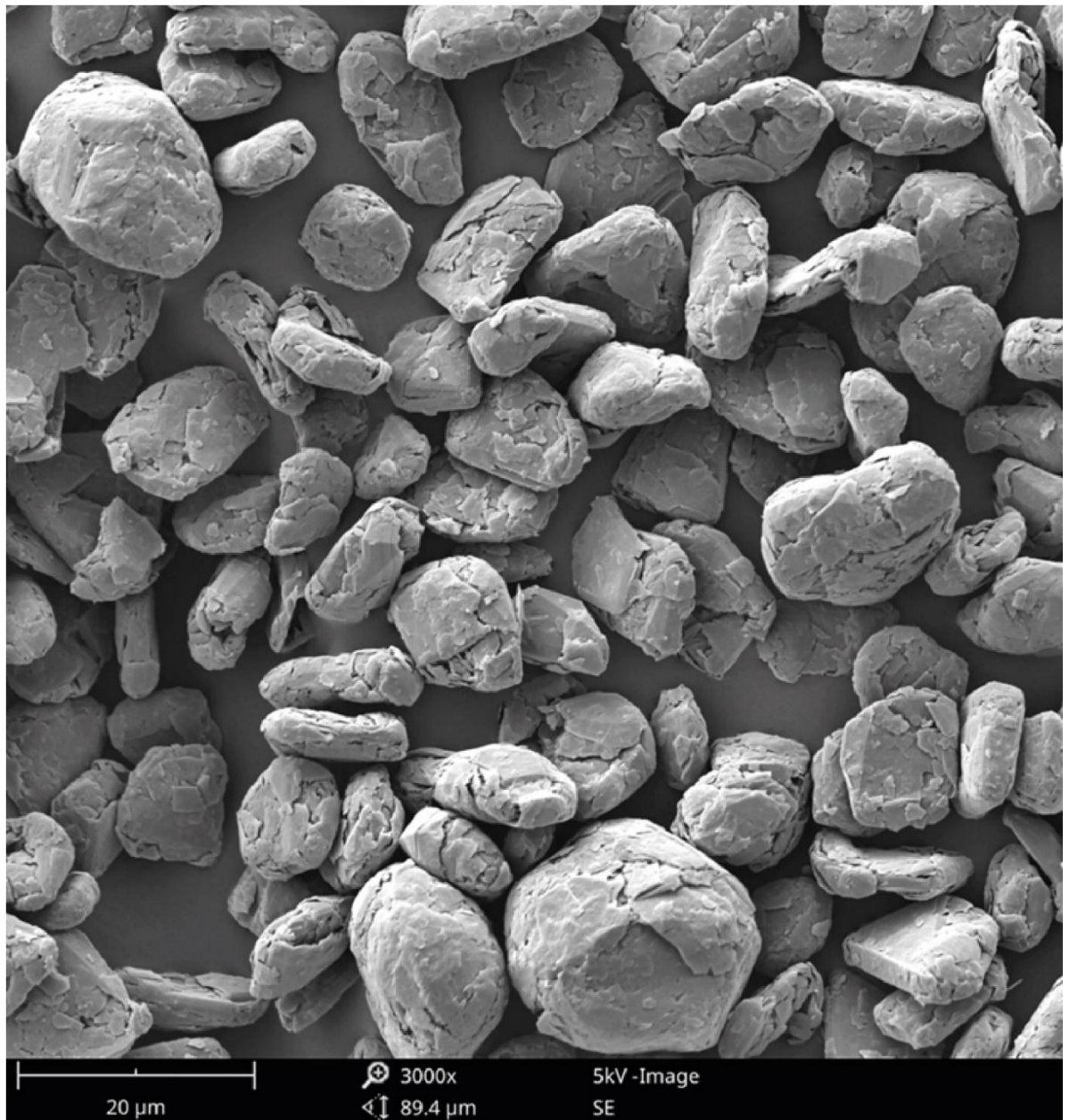
Figure 15: SEM image of reference material Ref 10; magnification 3,000x
