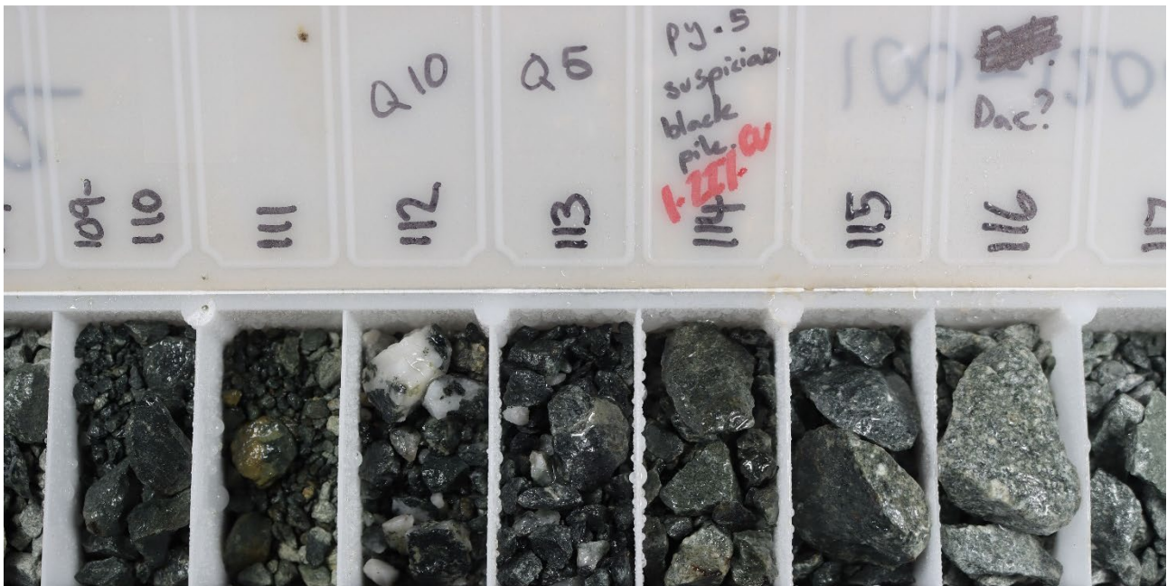
Figure 7: RC21KP1012 with 1m @ 0.52 g/t Au, 1.22 % Cu and 7.99 g/t Ag from 113m. Mineralisation is associated with sulphides and is situated within the bedrock and is interpreted to be the Gift Structure and not related to a paleochannel setting.
