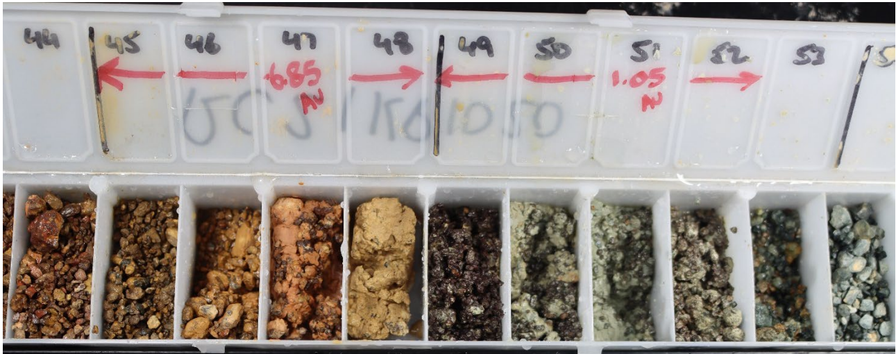
Figure 6: Oxidised quartz-gravel and clays within RC21KP1020 situated at the contact with saprock. Composite grades are written on chip trays. 1m re-splits of samples recorded 2m @ 7.89 g/t Au, 0.19 % Cu, 0.35 g/t Ag from 44m including 1m @ 14.40 g/t Au from 44m.
