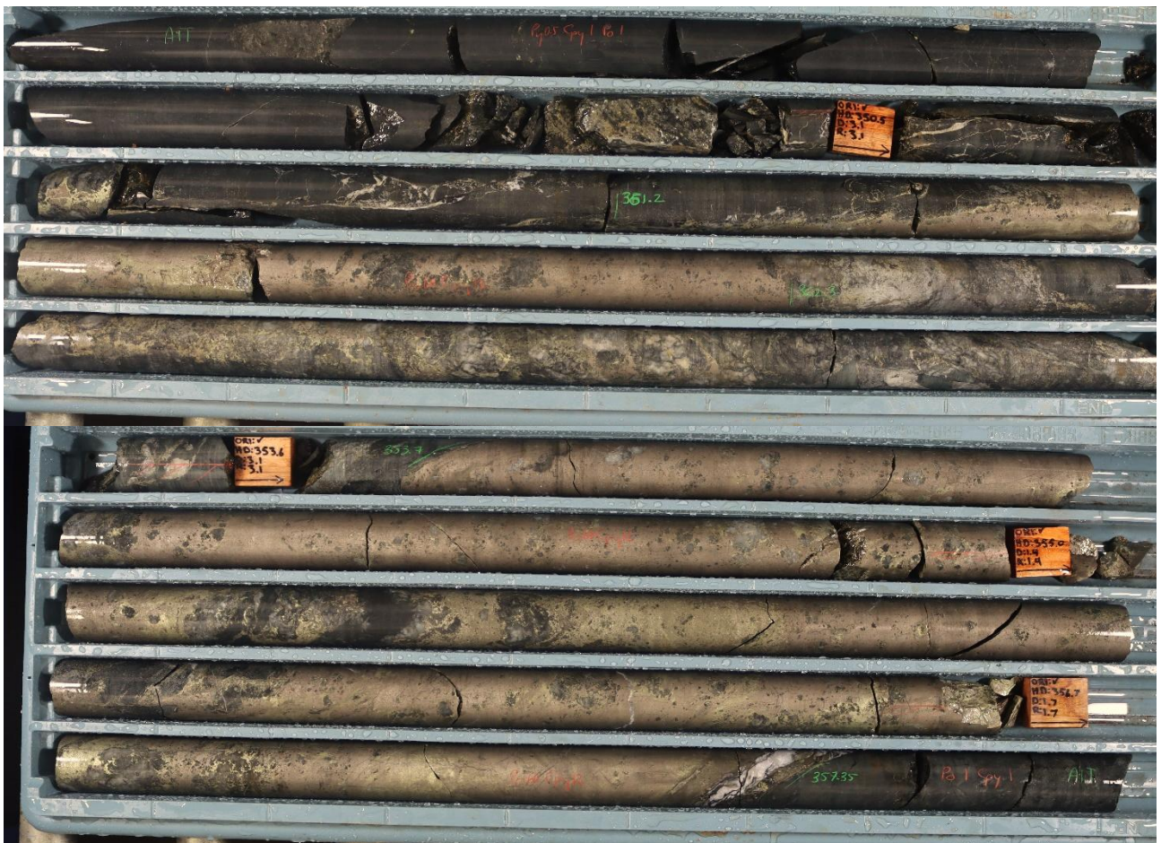
Figure 6: DD24KP1232 - ~6.65m interval of massive and semi massive sulphides overprinting quartz veining from 351.2m, comprised of pyrrhotite (60%) and semi massive chalcopyrite (15%) and pyrite (5%). True width of the interval is estimated to be approximately 65% of the visually logged intercept length based on. Refer to Annexure 4 for further information about orientation of data relative to geological structure.
