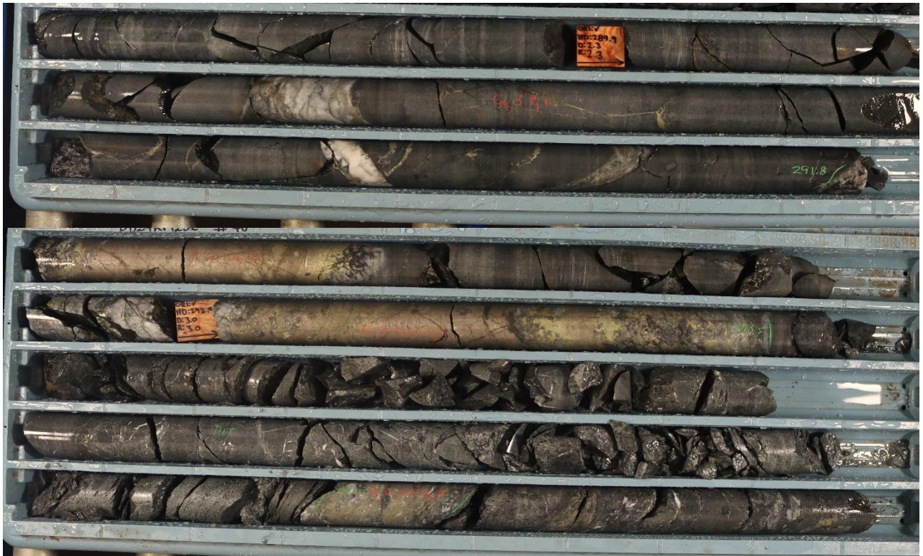
Figure 5: DD24KP1232 - ~1.7m interval containing two quartz sulphide veins from 291.8m comprising massive pyrrhotite (60%) and semi massive chalcopyrite (20%) and pyrite (5%) within an intermediate volcanic host rock.
