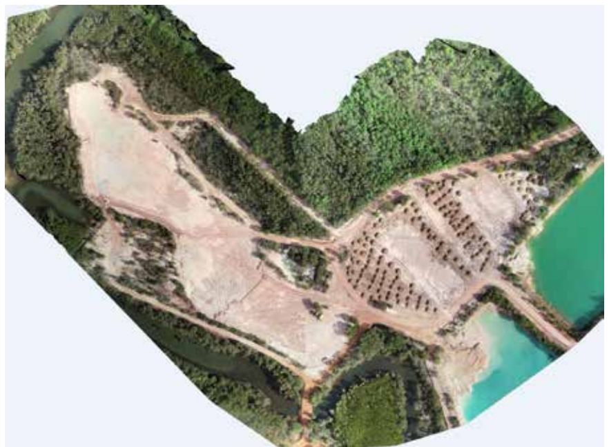
Before and after images of the fluvial pit and fluvial overburden rehabilitation. Note in the lower image the topsoil was in the process of being paddock dumped in preparation of spreading and seeding.
