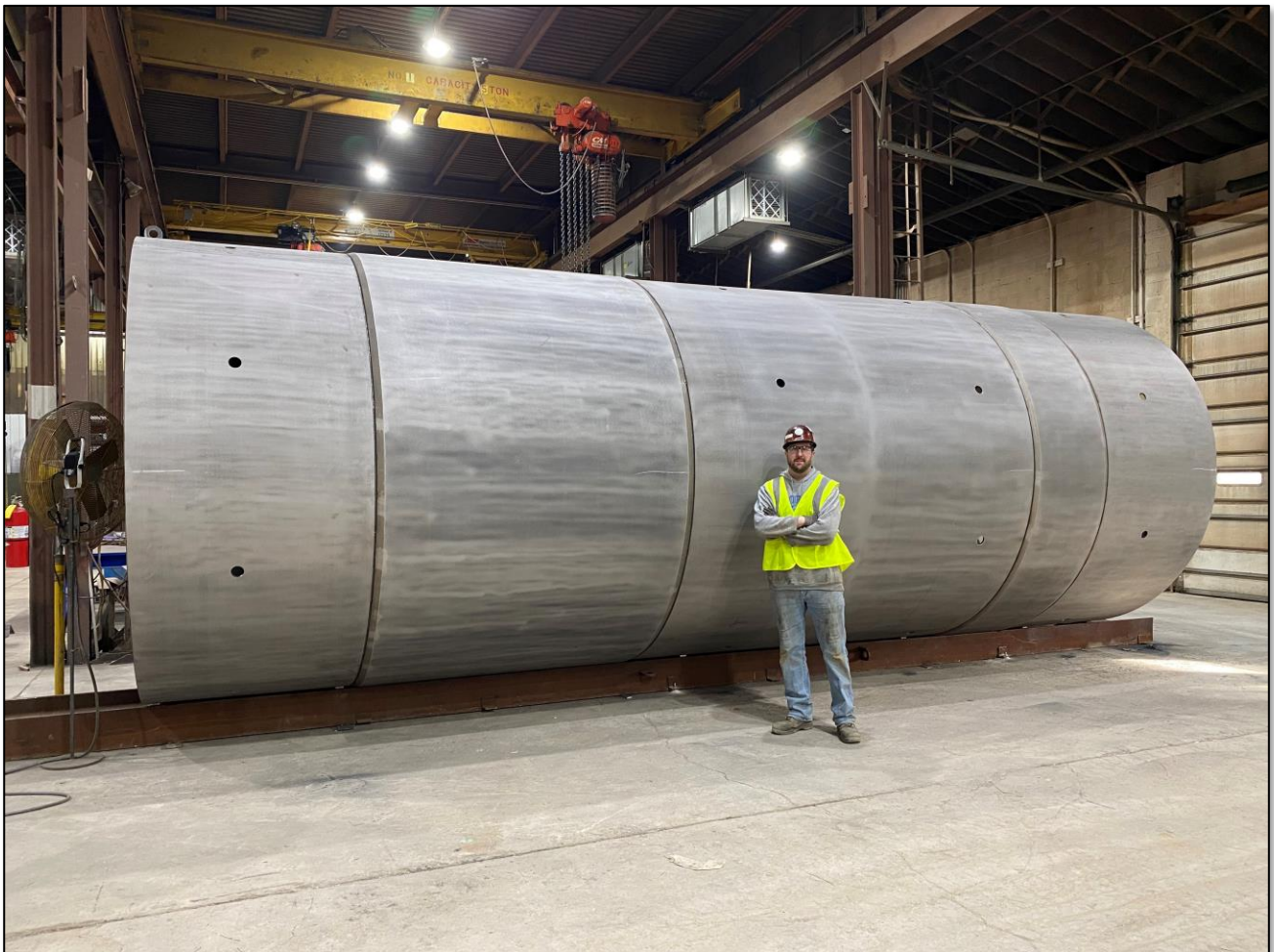
Figure 2 - FEECO Headquarters, Cabinda Phosphate Fertilizer Granulator Drum.
