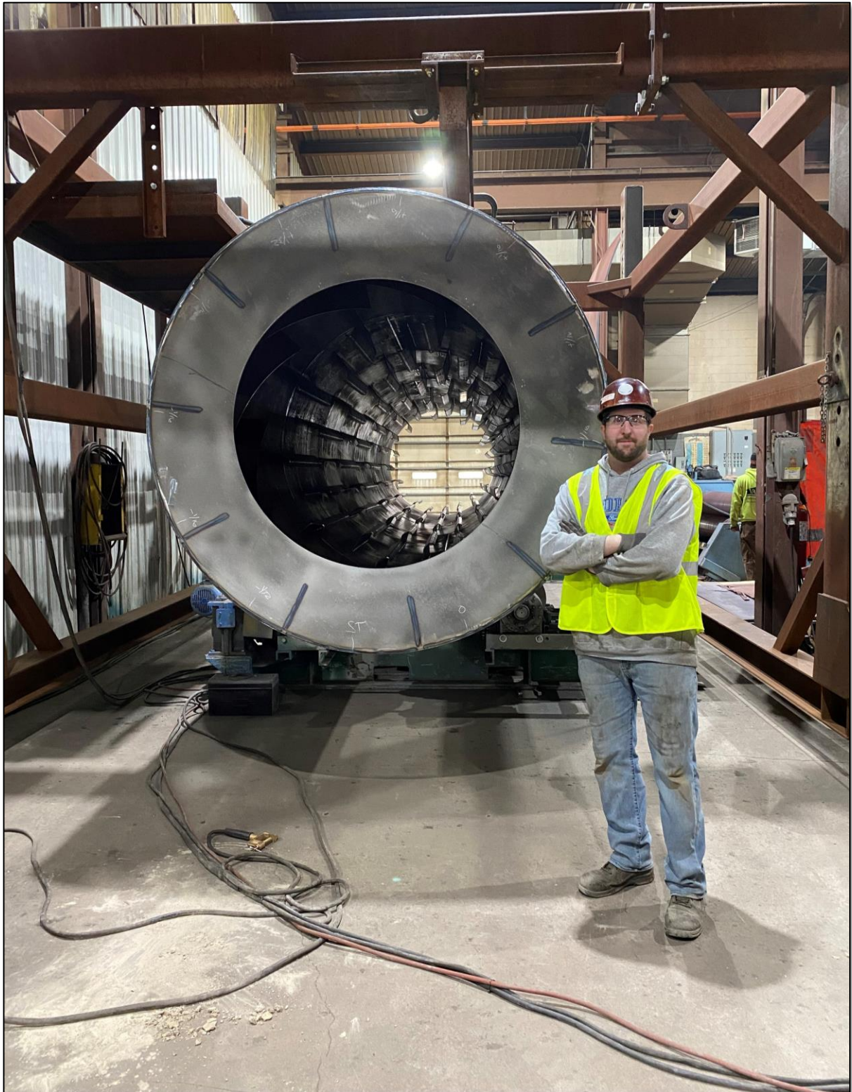
Figure 3 - FEECO Headquarters, Cabinda Phosphate Fertilizer Granulator Drum.
