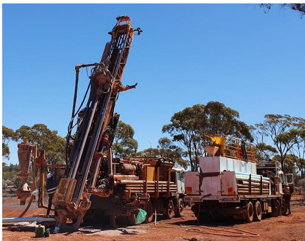
Figure 1: RC rig set up for drilling at Omrah nickel prospect
