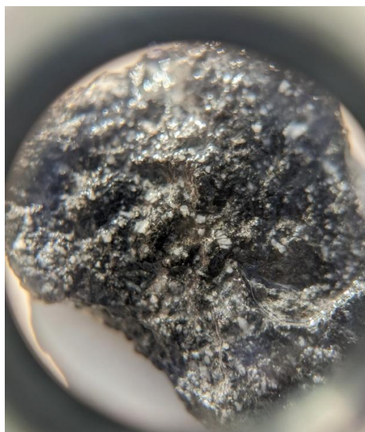
Figure 1: Dukes Hole SSMH0150 – sample within 20m of 5% to 10% sulphides
