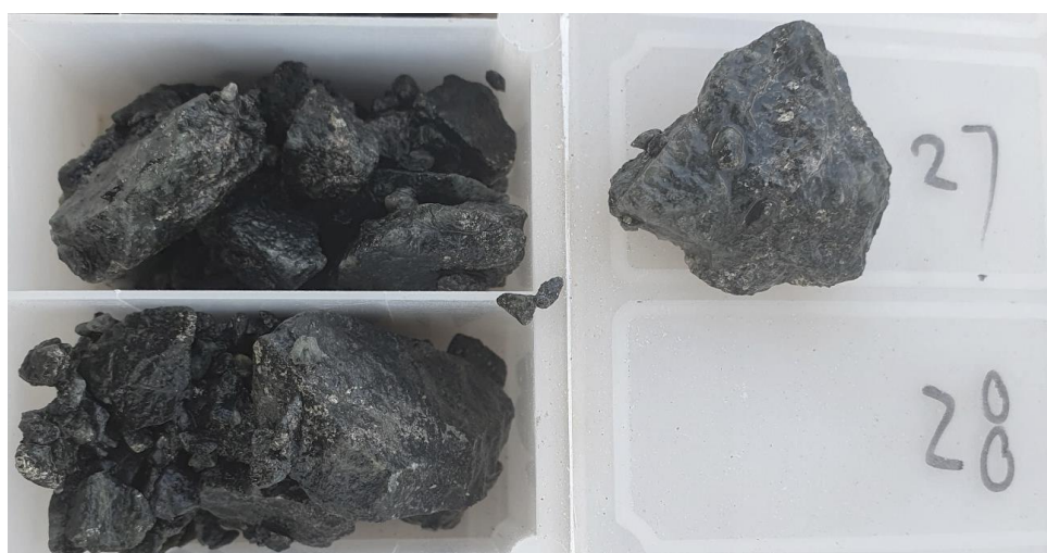
Figure 3: BCRC011 - Chip tray interval at 26m to 28m drill depth within a 5m interval of Intense Magnetite-pyrite-epidote skarn alteration from 24m depth at the upper contact of a skarn with decreasing magnetite and pyrite content and variable epidote- +/- garnet mineralogy to 60m depth.
