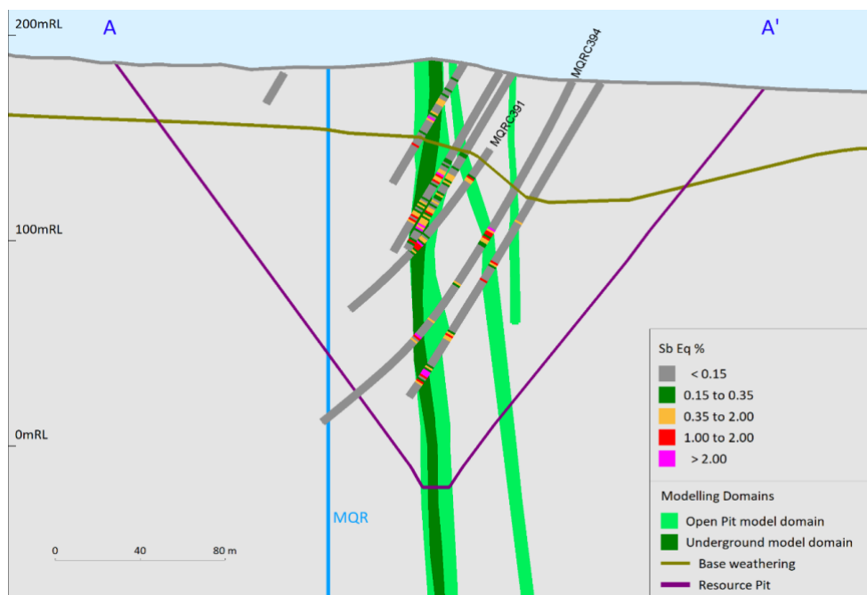
Figure 5 – A-A' section view facing east with open pit and underground domains illustrated with projected one metre downhole assays. Conceptual MQR open pit shell also projected onto section.
