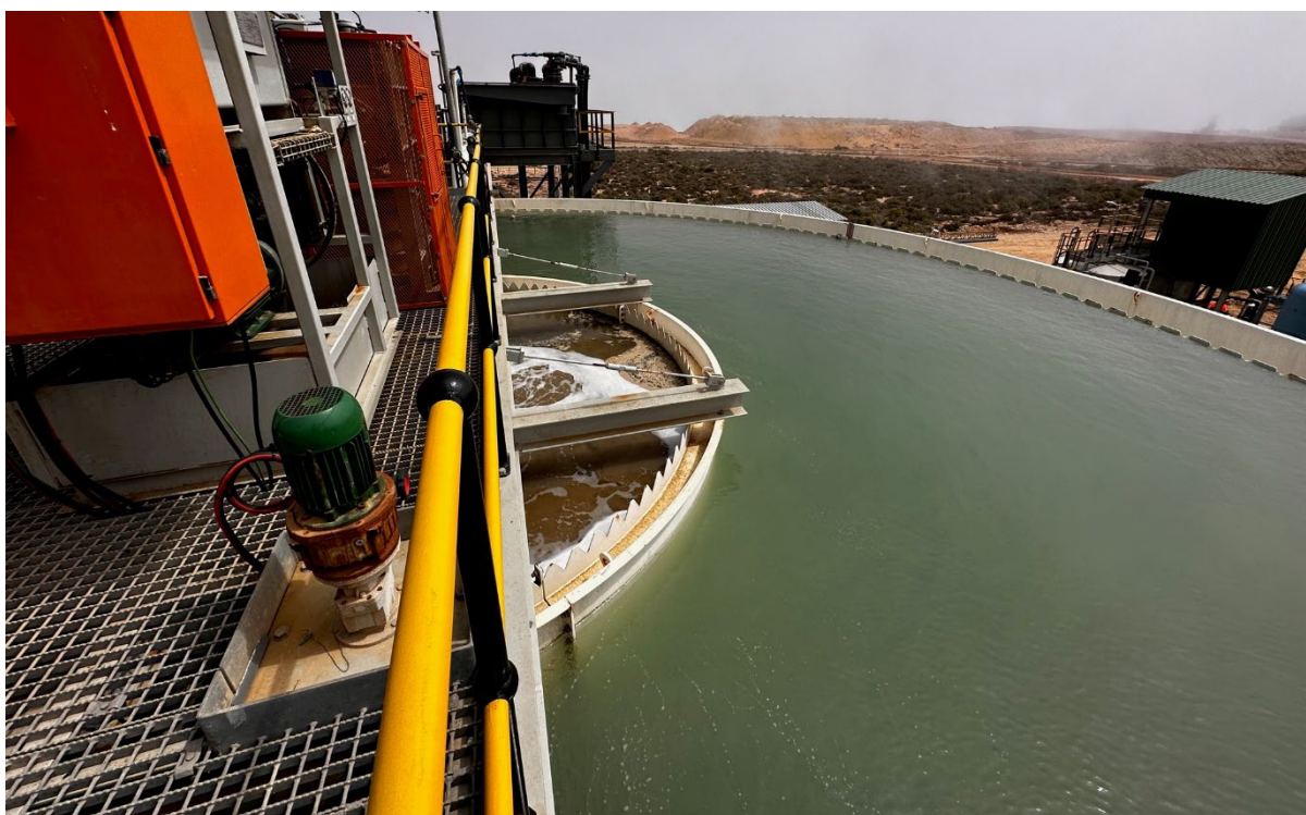
Figure 1 View from on top of thickener, showing well flocculated central feed well and clear overflow
