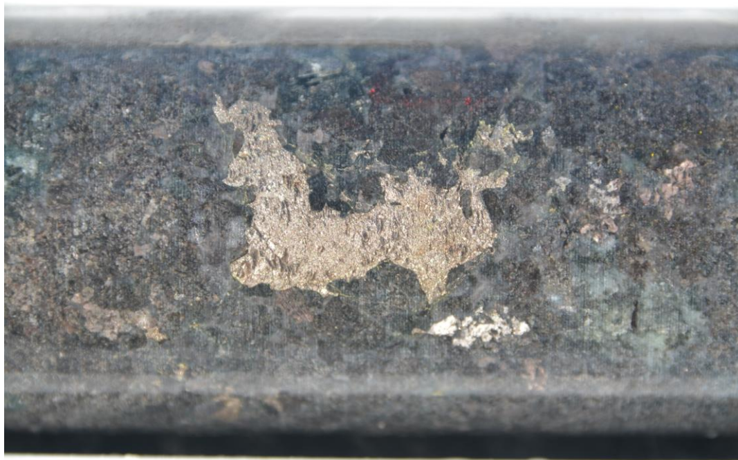
FIGURE 2: Core from MRDD011 showing blebbly sulphides at depth 211.20 metres. Portable handheld Niton XRF readings range from 1.9% up to 3.9% nickel and from 0.1% up to 1.7% copper.
