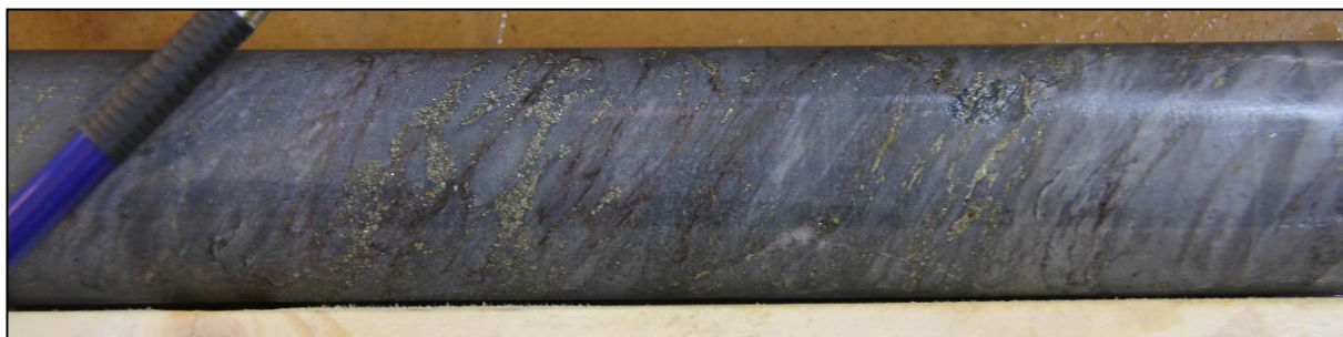
Figure 3: Pyrrhotite, pyrite and sphalerite mineralisation in intensely-altered felsic volcano-sedimentary rock. NOR17001, 46.5m.
