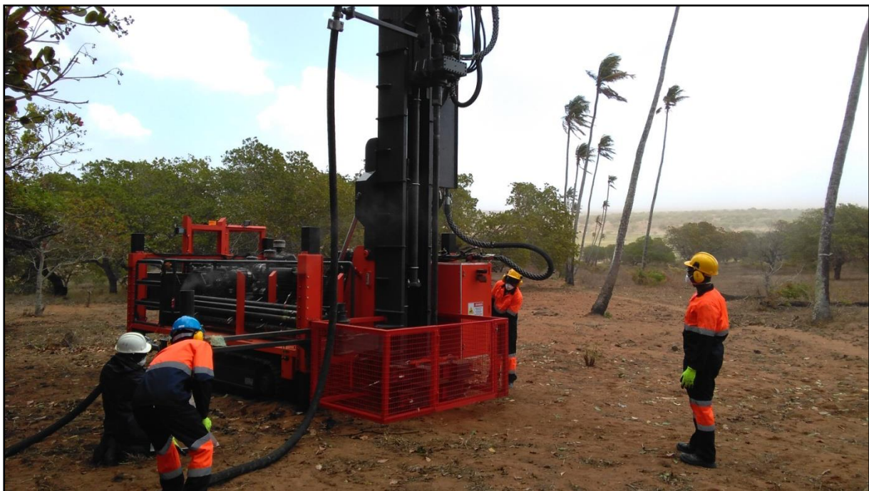
Figure 3: Aircore Drill Rig commences drill program at Koko Masava.
