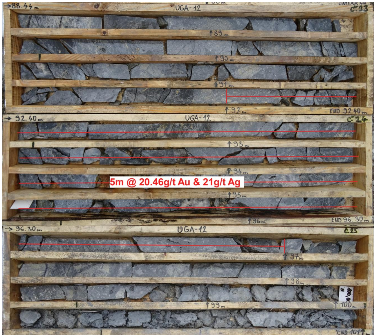
Figure 1: UGA-12 drill core; interval from 92m to 97m (down-hole) with assay grade 5m @ 20.46g/t Au and 21.0g/t Ag
