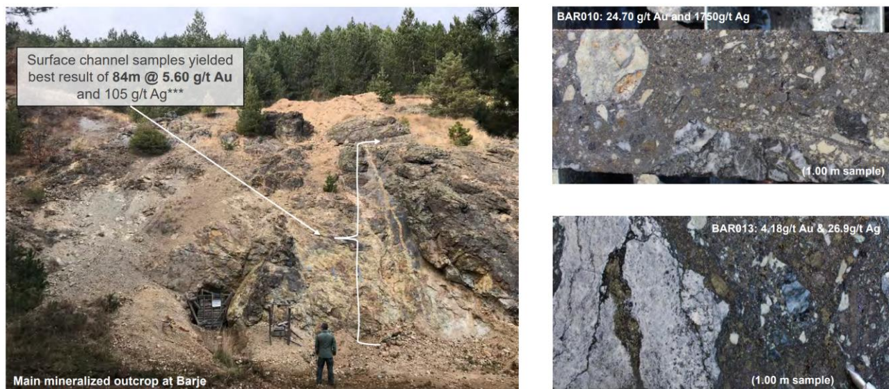
Figure 3, 4 and 5: Exploration undertaken at the Tlaminio Gold Project. Figure 3 (left) - channel sampling at the main mineralised outcrop at Barje (Tlaminio Project); Figure 4 (right, top) - core sample from drilling in hole BAR010; and Figure 5 (right, bottom) - core sample from drilling in hole BAR013
