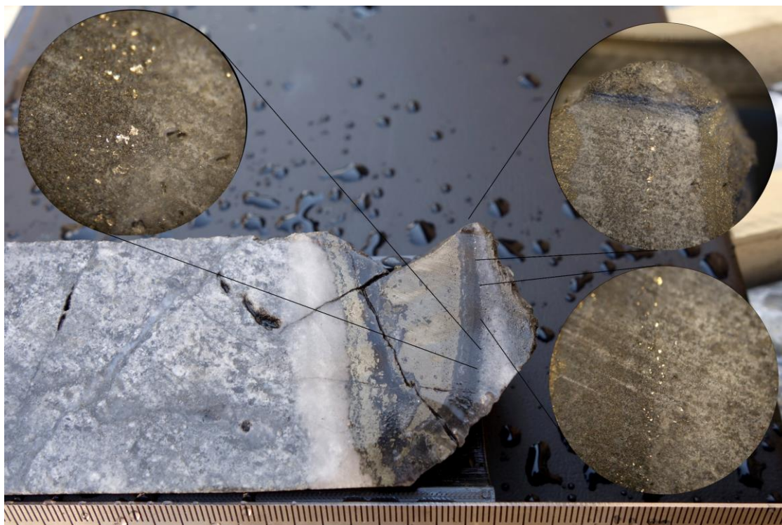
Figure 1: On this cut surface the Visible Gold is preserved as upto ~0.2mm sized grains within a ~5cm wide, grey-white, drusy quartz veinlet filled by fine-grained disseminated to semi-massive pyrite/marcasite crystals at 130.4m in UGA-41. Field of view of the right two magnified inset images is ~10mm across (x20) and the field of view of left magnified inset image is ~4mm across (x40).
