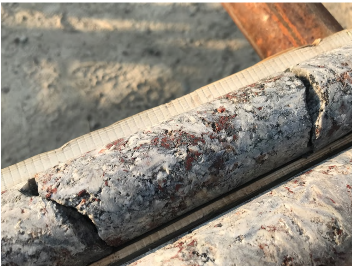
Figure 5: Diamond drill core (NQ, approximately 4.8 cm diameter) containing REE mineralisation (red coloured disseminations) within ferrocarbonatite host rock. Hole POM-23-01, Box 104, 475.6 – 479.9 metres downhole depth.
