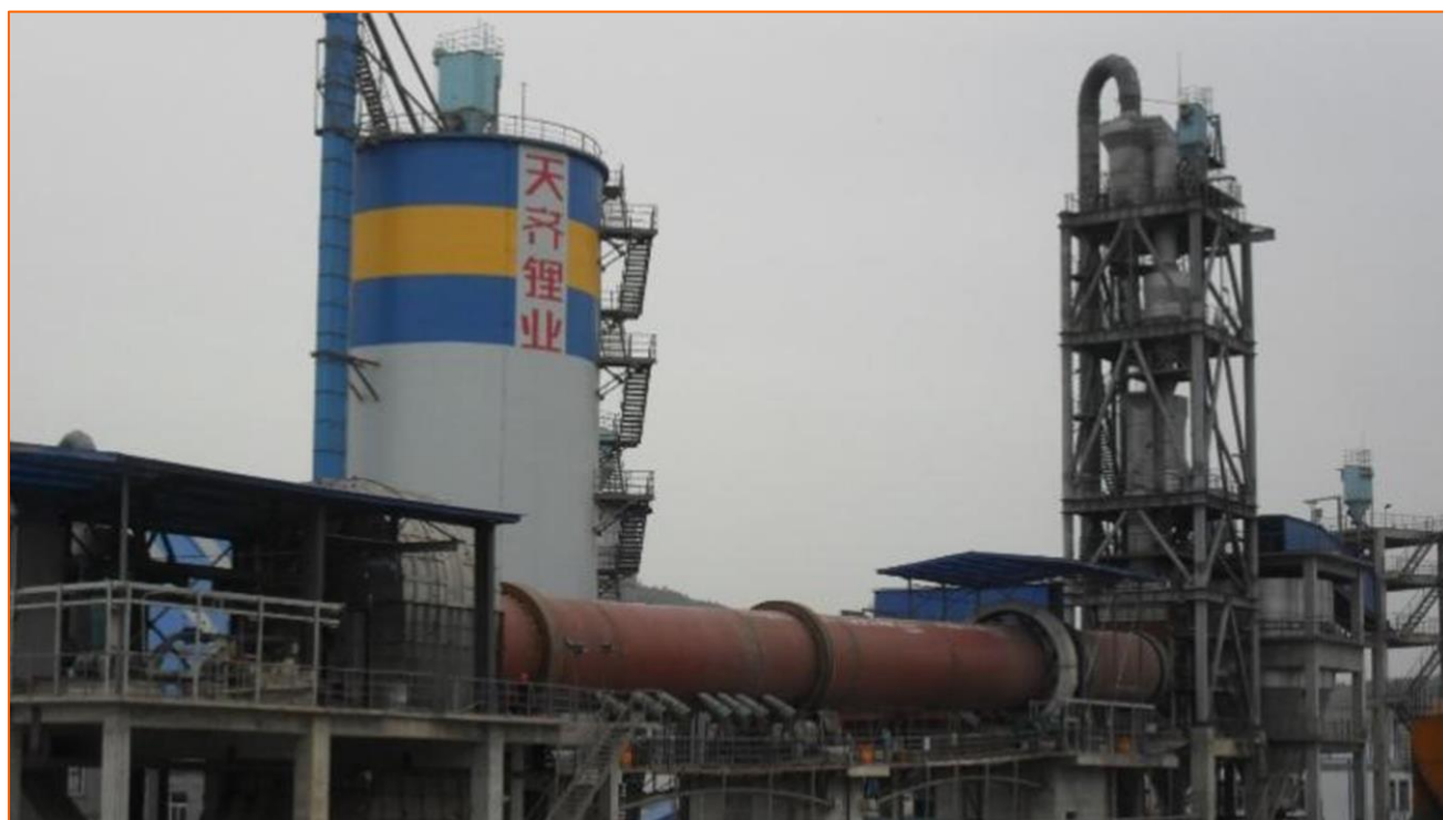
Figure 6: Typical natural-gas fired calcination kiln used in the lithium refinery process. Source: Sichuan Calciner Technology Pty Ltd
