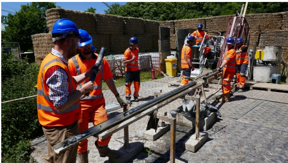
Exploration Manager, Brett Grist examining drill core pushed from the core barrel during drilling at Redmoor in May
