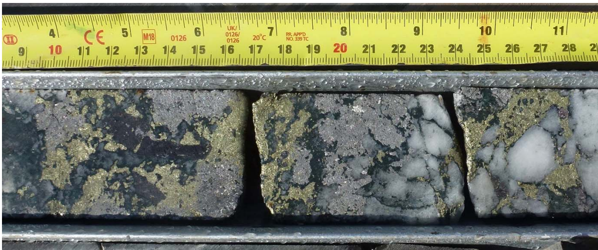
Figure 4 – CRD024: 589.5m –wolframite and chalcopyrite in quartz veins
