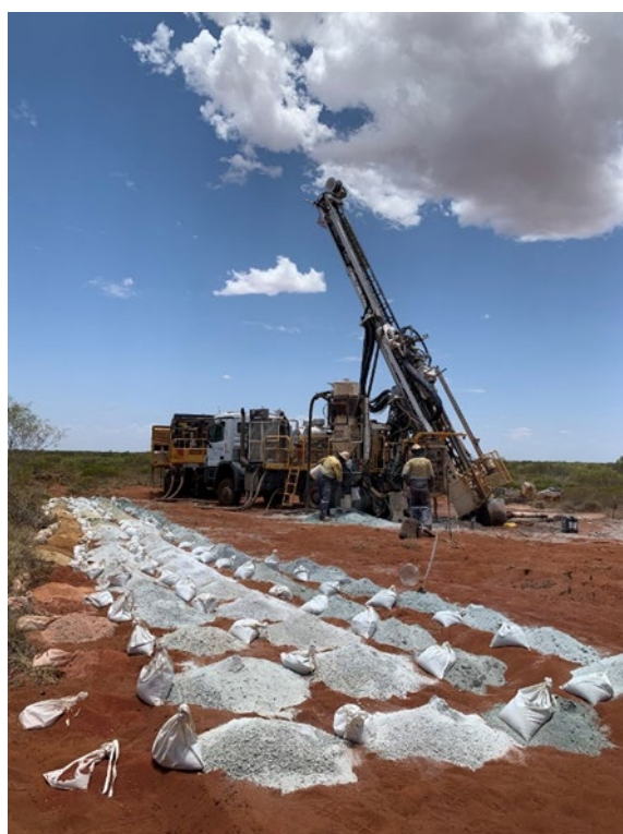
Photo 4: Strike Drilling T450 Aircore/Reverse Circulation Rig
