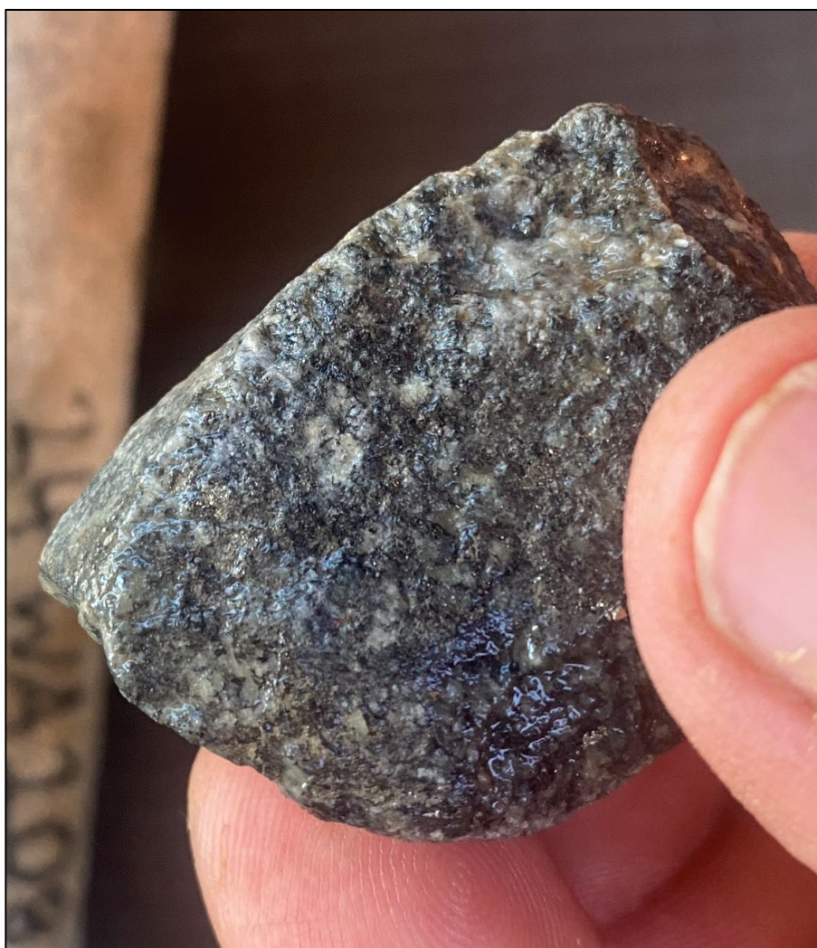
Figure 5: Interpreted intermediate intrusive rock with euhedral pyrite from drillhole 24WA108, Target 6.
