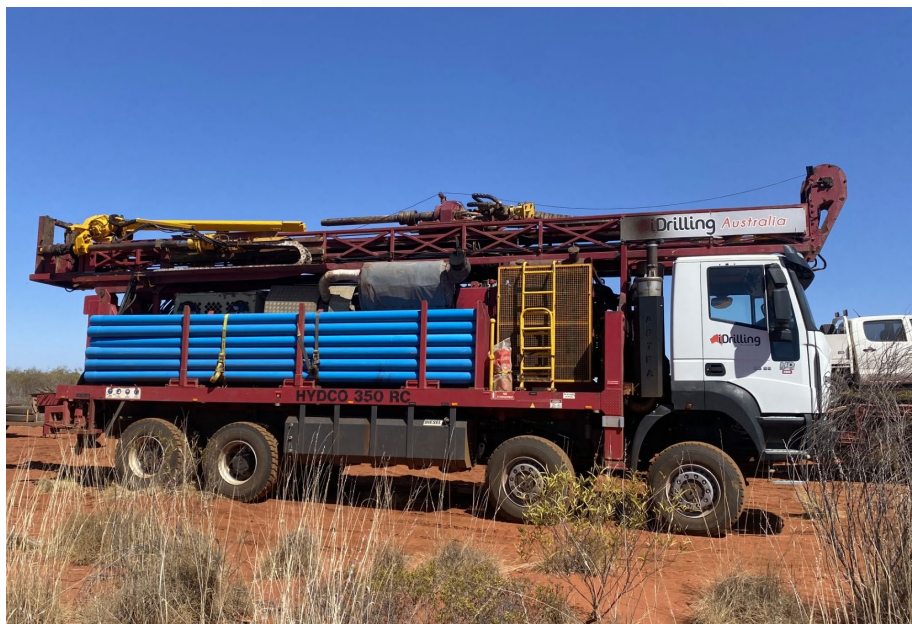
Figure 1: RC drill rig at Wagyu Gold Project
