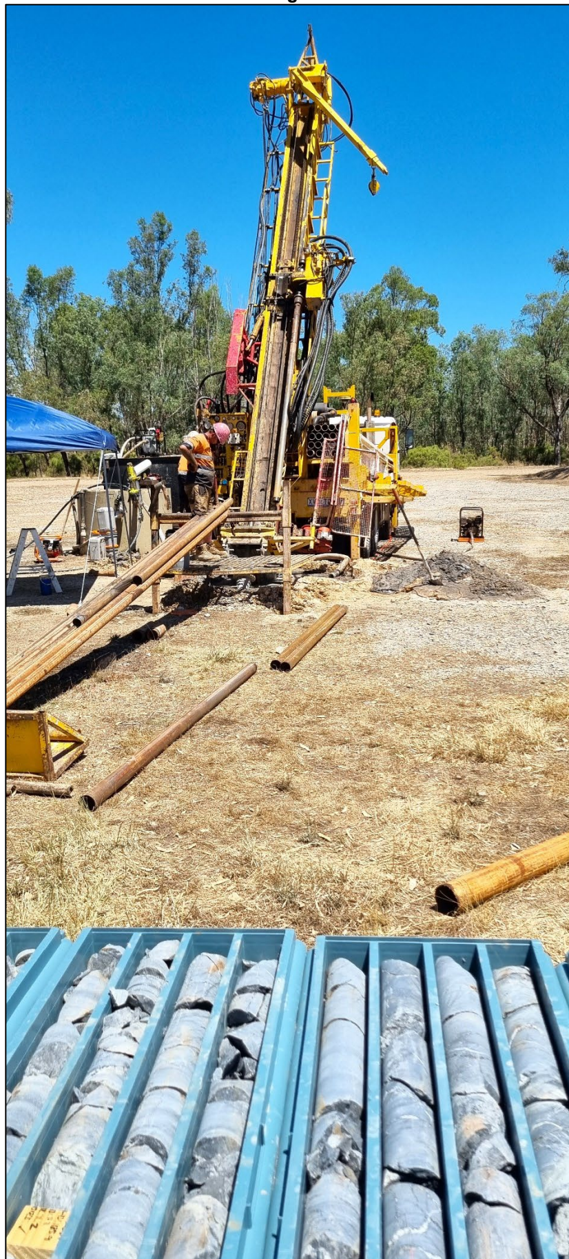
Photo 1 GMP Exploration Drilling Rig at the Nagambie Mine - Drill Core in the Foreground
