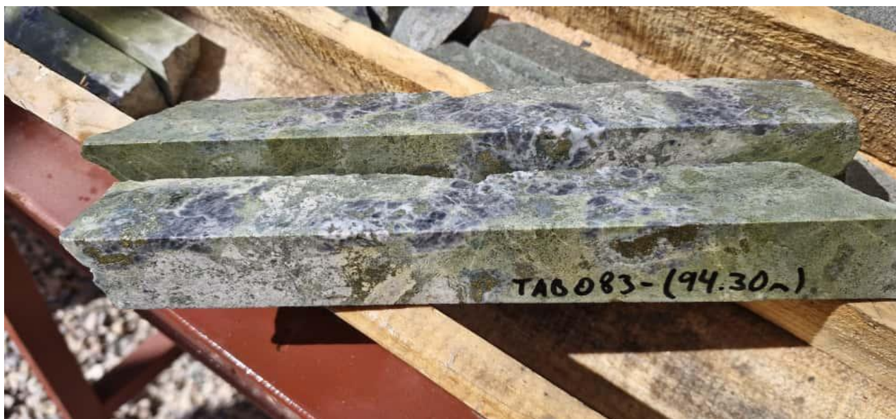
Image 7: Example of quarter core samples to be re-submitted for analysis
