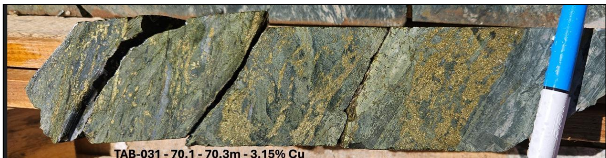
Image 6**: TAB 031 showing flow banded meta-sediment containing mainly Cu sulphides (Chalcopyrite) and minor pyrite
