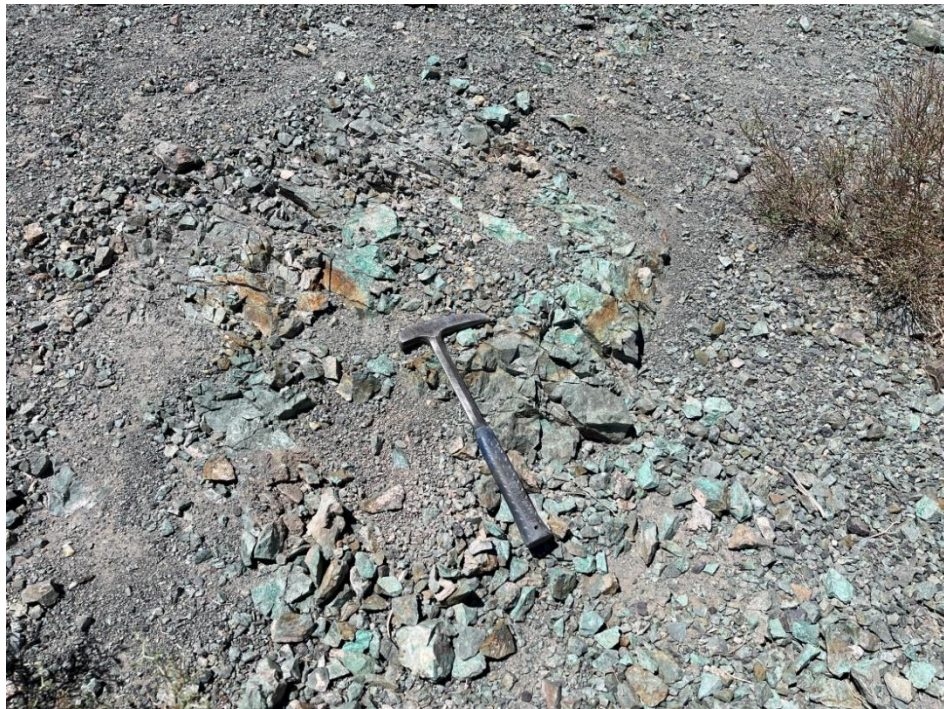
Image 4: Extensive Cu Oxide mineralization in fractured outcrop volcanic breccia host
