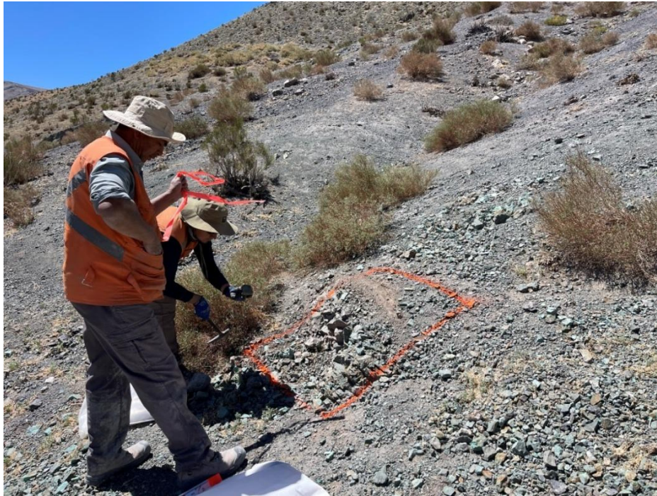
Image 3: Panel sampling over 2m x 2m across mineralized outcrops
